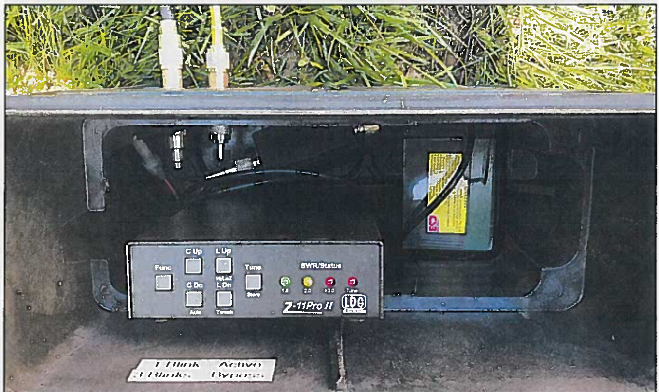
Photo C. Auto-tuner with battery and 1:1 choke in a gasketed ammo box.
